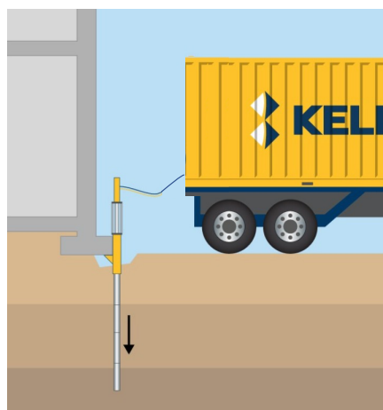
Figure 6 - Pile Jacking technique, as per Keller USA Limited
